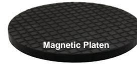
Magnetic platens combine a standard aluminum platen with a cross-hatched magnetic surface for maximum flatness and adherence. Only one platen is needed throughout the grinding and polishing process, allowing all magnetic system cloths/abrasive discs or ferromagnetic discs to be utilized.
