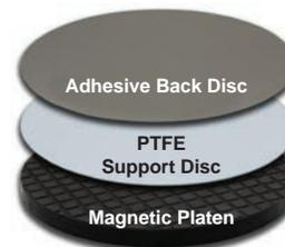
These reusable, durable discs combine a PTFE surface with a ferromagnetic stainless steel substrate. This allows adhesive backed abrasive discs/polishing cloths to be easily removed after use without any adhesive transfer. The nonslip backing keeps the disc in place, even for coarse grinding applications.
