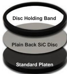
Disc holding bands are made of anodized aluminum and secure plain back discs to a standard platen. A protrusion around the top of the band allows variable sized discs ( $\pm 3$  mm) to be secured.
